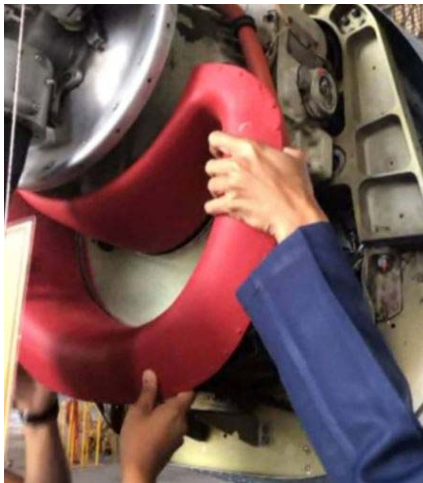
INLET AIR DUCT
